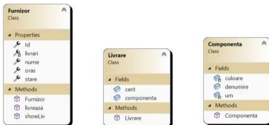
Figure 6. UML Style Class Diagram Auto-Generated by Visual Studio's Dedicated Component
