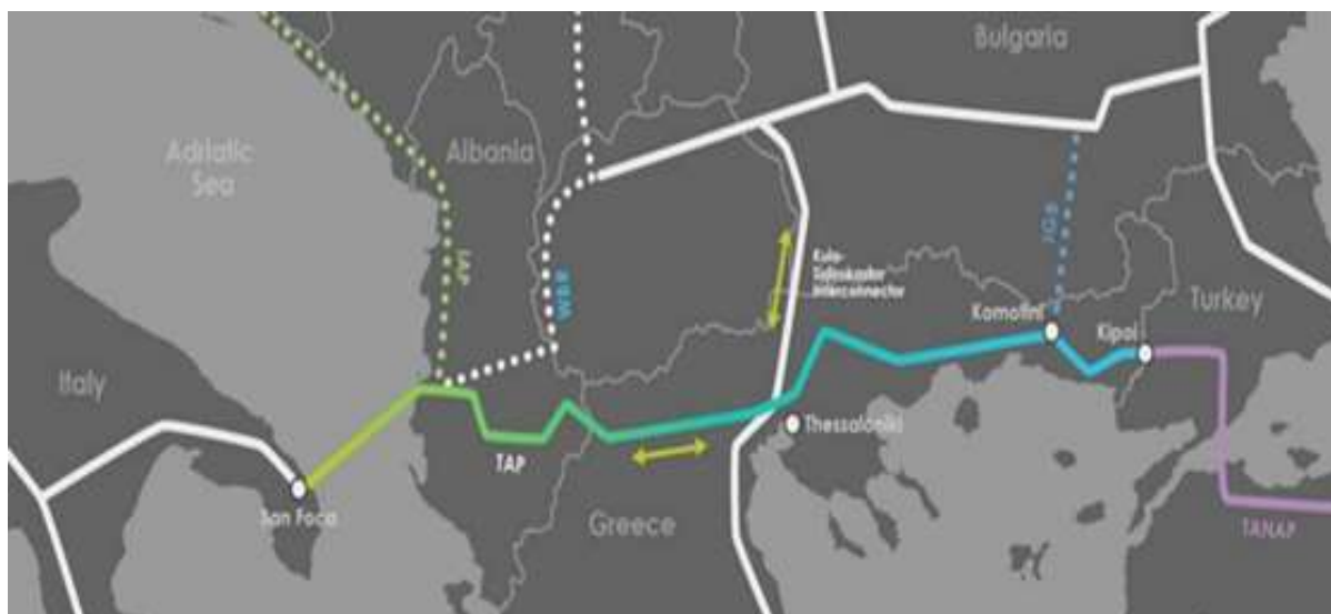
Figure 1. Map of the Trans Adriatic Pipeline (TAP) and its connection to Europe's NG network
